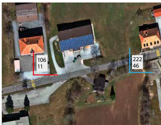
An aerial image with sample points and codes indicating the determined land use. Code 106/11 stands for "consolidated surface in public building area".
