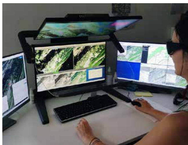
An analyst interpreting the aerial photos on a stereoscopic 3D monitor. The two side screens display additional information.
